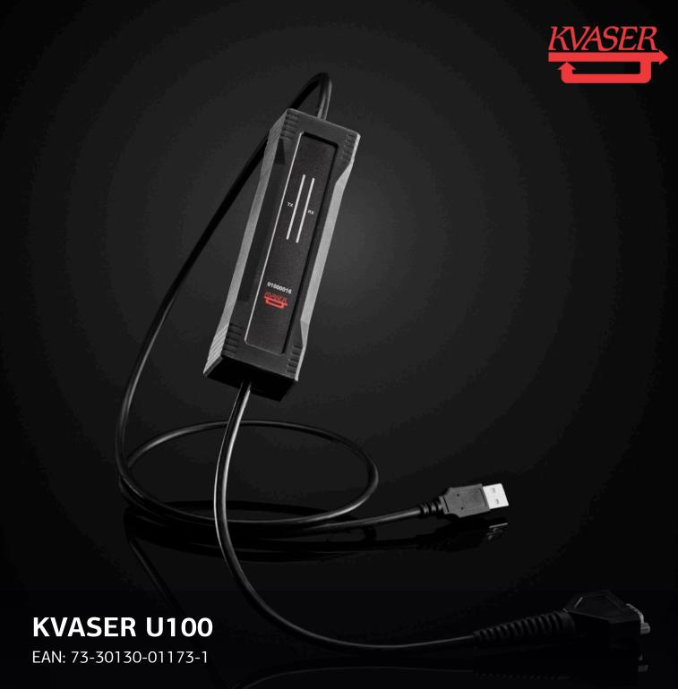
The Kvaser U100 is a robust, single-channel CAN/CAN FD to USB interface with reinforced galvanic isolation (Tested according EN 60335) that squarely addresses the needs of the evolving automotive development market. Fully compatible with J1939, CANopen, NMEA 2000® and DeviceNet, this is the first in a new range of interfaces that is also suited to rugged applications in marine, industrial, heavy duty vehicle and heavy industries.
