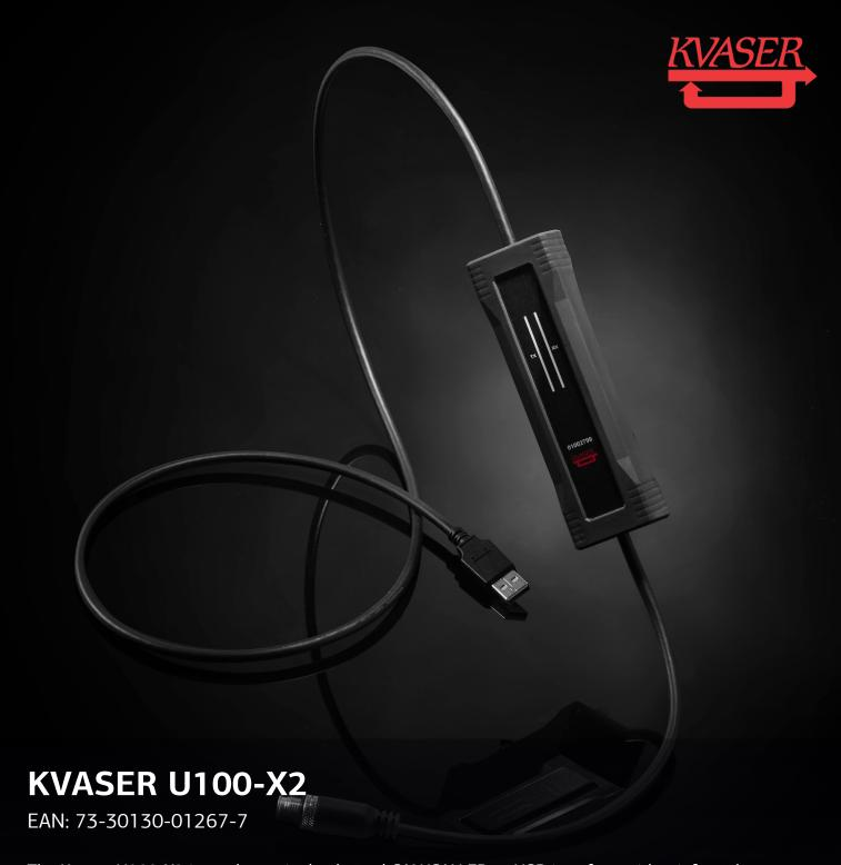
The Kvaser U100-X2 is a robust, single-channel CAN/CAN FD to USB interface with reinforced galvanic isolation (Tested according EN 60335) that squarely addresses the needs of the evolving automotive development market. Fully compatible with J1939, CANopen, NMEA 2000® and DeviceNet, this is the first in a new range of interfaces that is also suited to rugged applications in marine, industrial, heavy duty vehicle and heavy industries.
