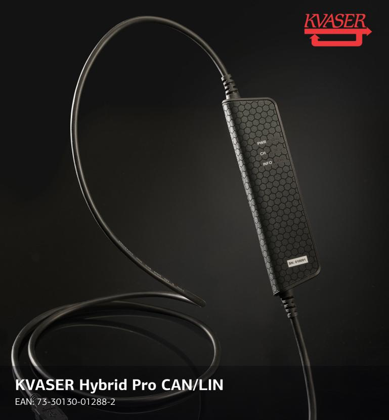
Kvaser Hybrid Pro CAN/LIN is a flexible, single channel interface that can be assigned as either CAN, CAN/FD or LIN. This makes the Kvaser Hybrid Pro CAN/LIN a must-have 'universal interface' for every engineer involved in automotive communications!
